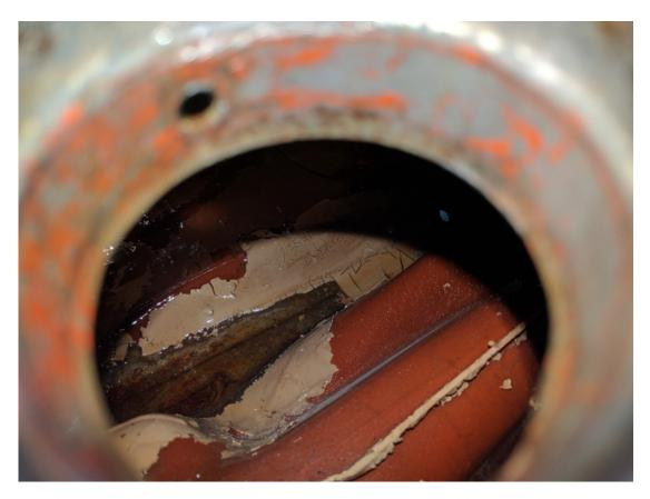
The original tank linings were never meant to withstand the ethanol levels found in current gasolines, and will peel away fairly quickly leaving uncoated areas subject to rust and corrosion. Especially in bikes that sit for extended periods with untreated gasoline in the tanks.
